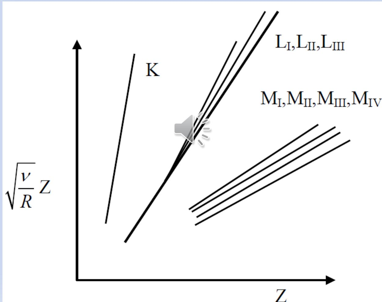
Moseley's diagram of X-ray absorption edges
