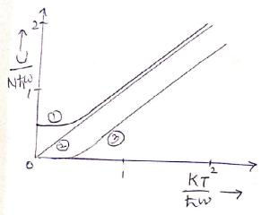
Just the figure, mean energy per oscillator is plotted as a function of temperature.
