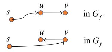
(u, v) is critical in  $G_f$  if (u, v) has the smallest capacity in augmenting path p in  $G_f$ .
