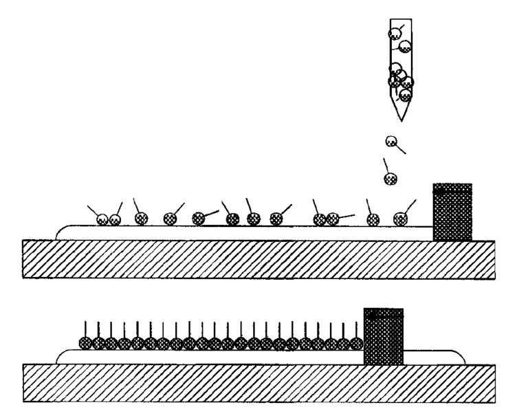
Schematic showing the formation of Langmuir films, which denote the molecular films at the water-air interface, a drop of a dilute solution of an amphiphilic molecule in a volatile solvent, such as  $CHCl_3$ , is spread on the water-air interface of a trough.
