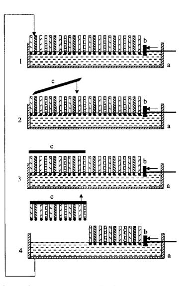
Schaefer's method useful for the deposition of very rigid films, in which, a compressed monolayer is first formed at the water and air interface, a flat substrate is placed horizontally on the monolayer film.
