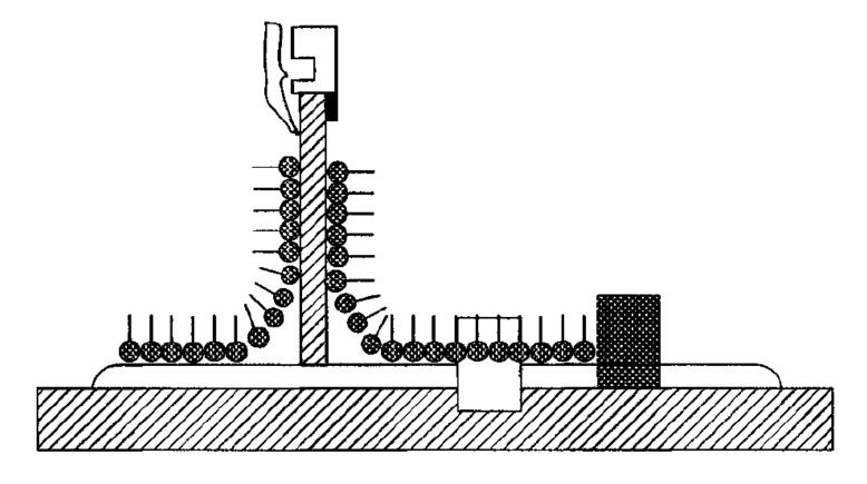
The more conventional vertical deposition method for the formation of LB films on substrates.
