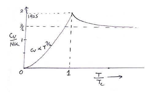
when T<sub>c</sub> is smaller than 1, a increases with femperature like  $T^{3/2}$  to a maximum value. At  $T=T_c$  a spike appears and when  $T\to\infty$  Cr approaches  $\frac{3}{2}$  NK, value
