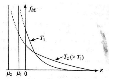
Plots of  $f_{BE}$  versus  $\varepsilon$  for bosons at two different temperatures  $T_1$  and  $T_2$  (>  $T_1$ )
