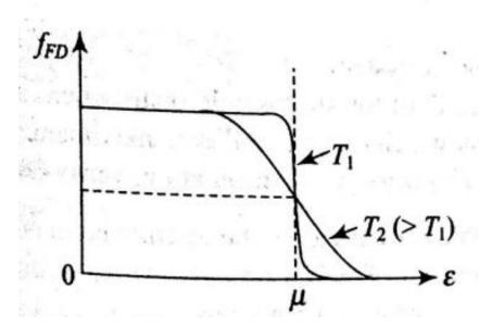
Plot of  $f_{FD}$  versus  $\varepsilon$  for fermions at two temperatures  $T_1$  and  $T_2$  (>  $T_1$ )
