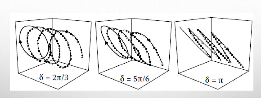
As the phase difference angle increases and reaches 180°, the minor axis become zero and also the polarization plane changes by 90°
